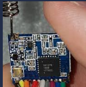
LoRa Module for Remote Launch Capability
